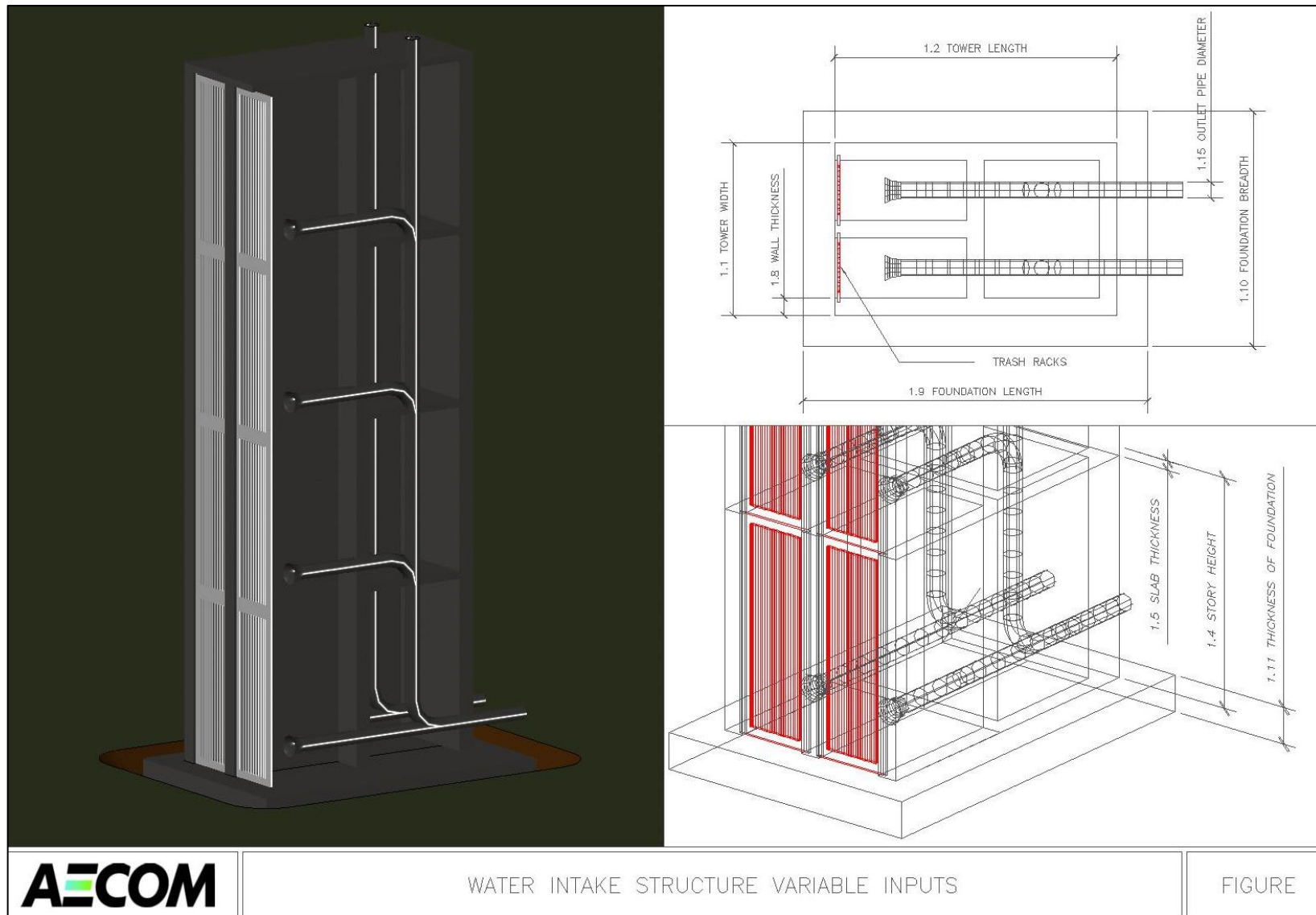
Figure 4.23: Water intake structure
